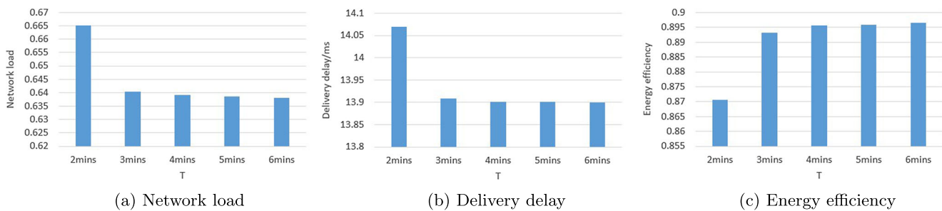
Fig. 11 The experimental results on network load, delivery delay and energy efficiency with chunk-level (100K)
