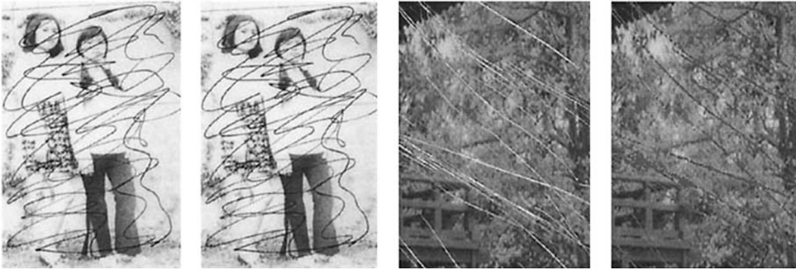
Photo Defect Detection. Figure 2. Damages from ink pen (a) are detected (b) Scratch (c) is detected (d).
